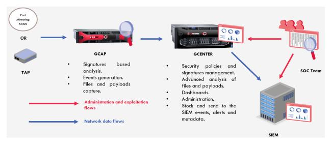
The Gatewatcher POC solution is based on 2 Dell R640 appliances server:
